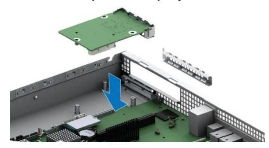
Figure 43. Intel ® I/O Module Placement
