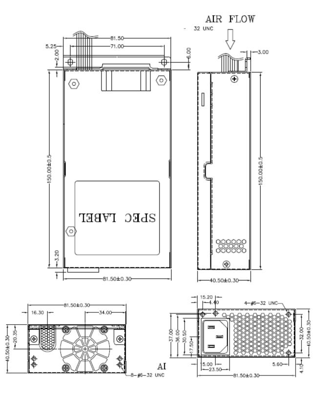
Figure 17. 400W Power Supply Mechanical drawings
