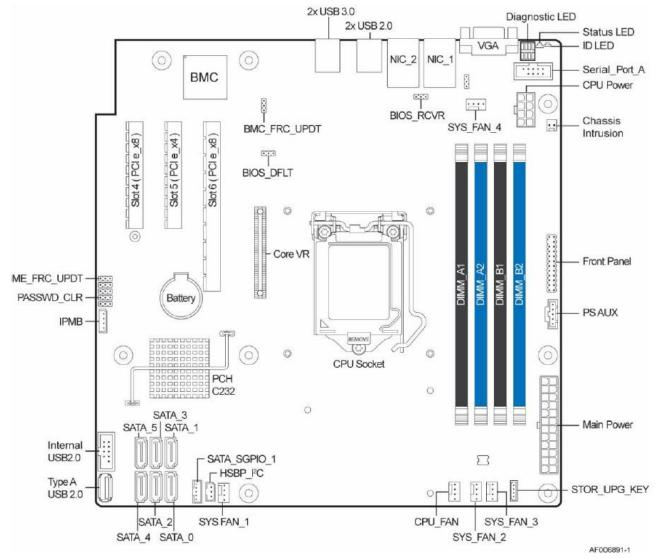
Figure 4.Server Board S1200SPS Features
