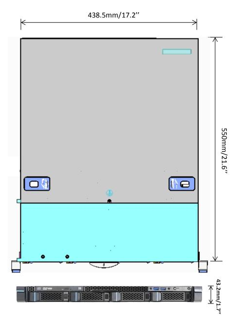
Figure 11. Chassis Dimensions
