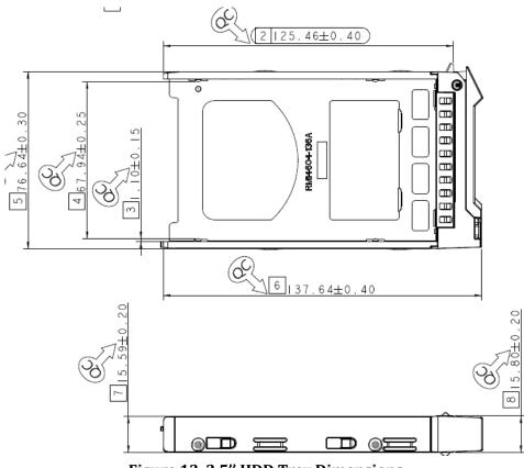
Figure 13. 2.5" HDD Tray Dimensions
