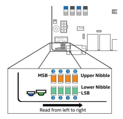
Figure 46. POST Diagnostic LED Location
