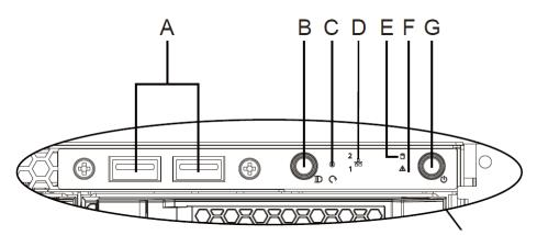
Figure 39. Front Panel Control and Buttons
