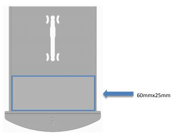
Figure 14. Pull-out Tag Label Emboss Dimensions
