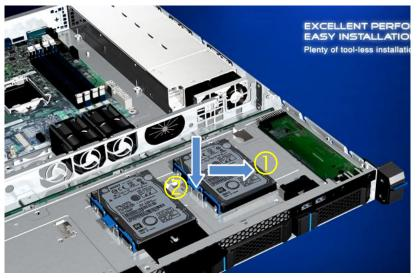
Figure 29.Internal 2.5" HDD Installation
