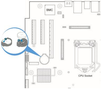
Figure 45. Replacing the Backup Battery
