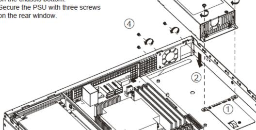
**Figure 16. Power Supply installation**
