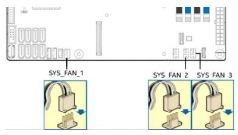
Figure 22.System Fan Connector Locations on Server Board
