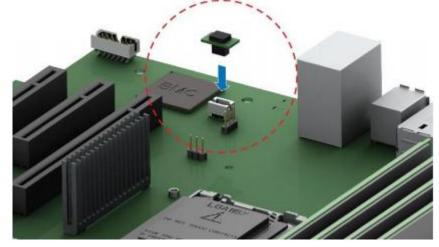
Figure 44. Intel® RMM4 Lite Activation Key Installation
