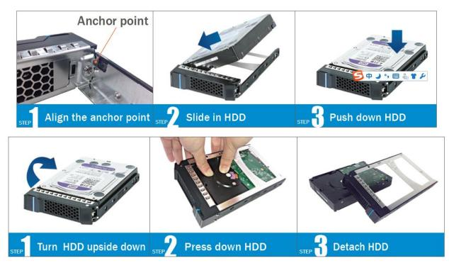
Figure 27.3.5"HDD Installation and Removal
