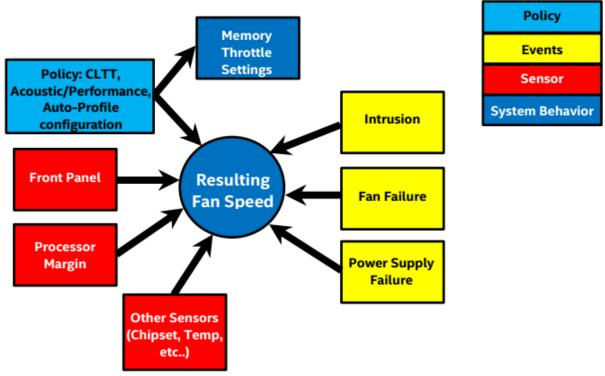
Figure 20.Fan Control Model
