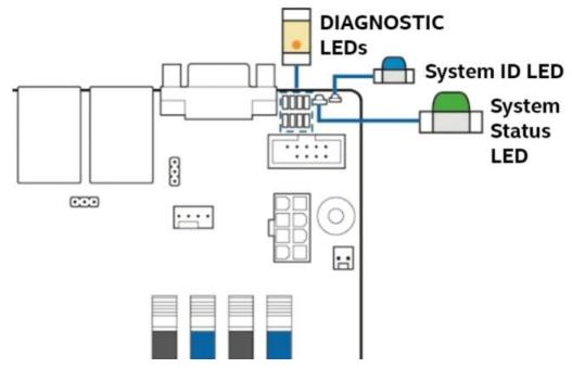
Figure 5.On-board Diagnostic LEDs
