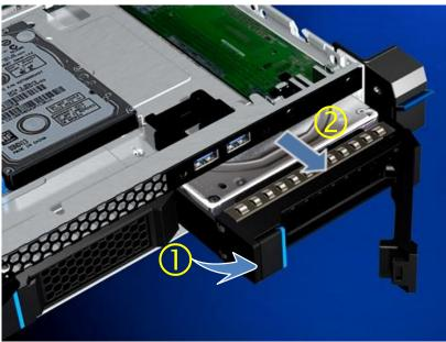
Figure 25. Hot Swap Storage Device Carrier Removal
