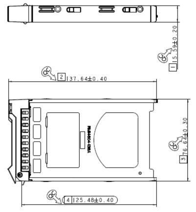
Figure 12. 3.5" HDD Tray Dimensions
