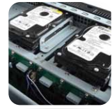
2 x 3.5" internal HDD bays
